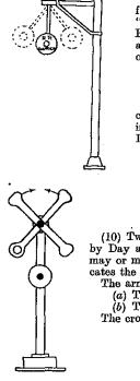
(9) An Arm carrying a Red Bauner swinging from a bracket and bearing in white the words "R.R., Danger" seen by day, or a Red Swinging or Flashing Light by night, signifies Danger, a train is approaching. A bell clangs when the signal is operating.
