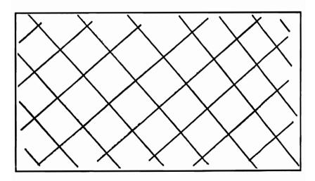
Size of diamond to be  $\frac{W}{9}$ , where W = the lane width. Width of lines to be 100 mm.
