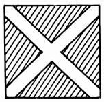
(b) When owing to the bad state of the landing area or for any other reason the observance of precautions in landing is required, there may be placed horizontally a red square panel each side of which measures at least 10 ft. and one of the diagonals of which shall be marked by a yellow strip at least 20 in. in width, as illustrated below:—
