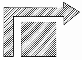
If, however, the only object of such suspension as aforesaid is that in such a case the landing area shall be kept on the right and that circuits or partial circuits shall be right-handed, the red square panel shall not be displayed.
